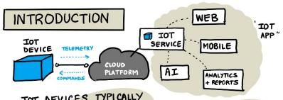
TOT DEVICES TYPICALLY CONNECT TO A SINGLE CLOUD IOT SERVICE - USING A STANDARD COMMUNICATION PROTOCOL
