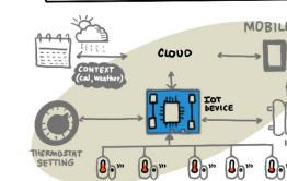
COMMANDS ARE: MESSAGES FROM CLOUD TO DEVICE WITH A REQUEST FOR ACTION ( ACTUATOR)
