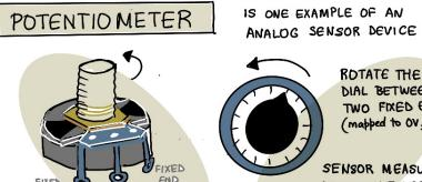
(mapped to OV, 5V) SENSOR MEASURES ROTATION BY SENDING REDUCED VOLTAGE (OR NUMERIC MAPPING) CORRESPONDING TO SHIFT
